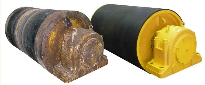
The pulley pictured was fully inspected at Dyna's modern workshop facilities which revealed – worn lagging, fatigued bearings, and damaged locking assemblies.
