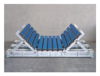
Impact beds are used in place of impact idlers/rollers and are installed under the belt at the loading points to absorb the impact from falling material.
