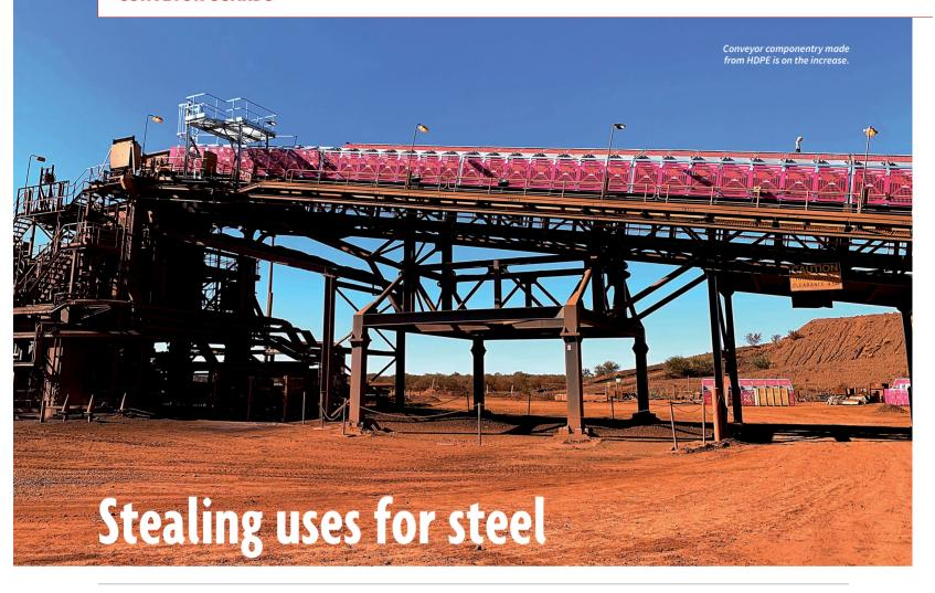
DYNA Engineering's HDPE (plastic) conveyor guards are providing Australian miners with a sustainable solution for site safety.
