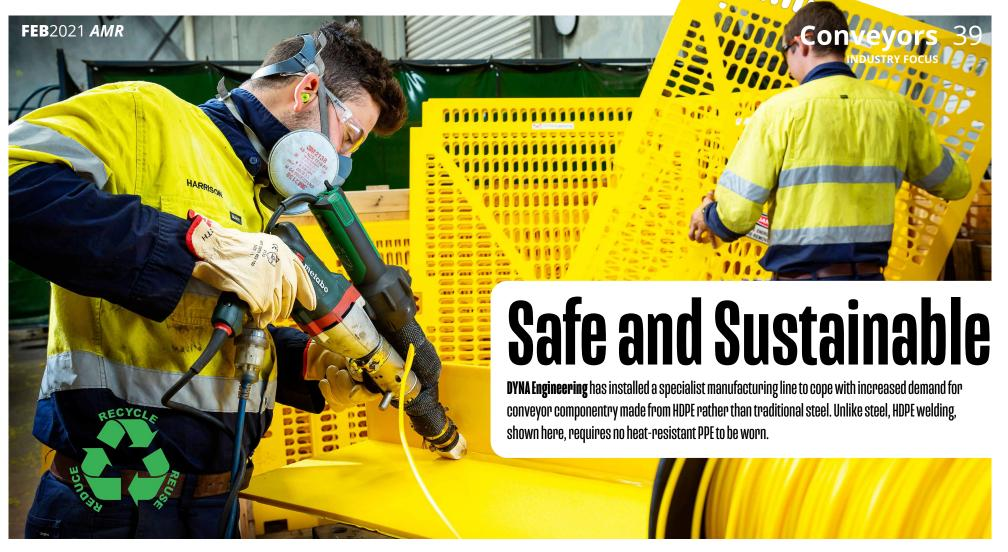
YNA Engineering's HDPE (plastic) conveyor guards are providing Australian miners with a sustainable solution for site safety.
